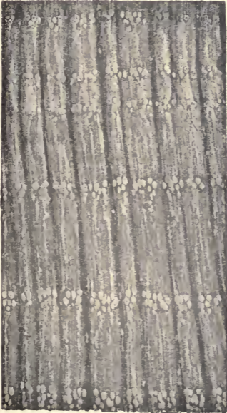
FIG. 38.—Transverse section of wood of oak (magnified five diameters), showing five annual rings, as denoted by the large vessels of the spring wood; the vessels become smaller in the summer and autumn wood, and are arranged in tongue-like groups. Nine broad medullary rays are shown, the rest are very narrow ( cf. fig. 27). The rest of the section is filled with tracheids, fibres, and wood-parenchyma. (Müller.)
